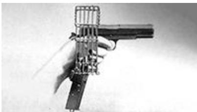
A nifty piece of aviation hardware turned up on the *National Rifle Association's* website in a 30 September 2022 post. An M1911 pistol fitted with the 'RFC Pistol Cartridge Case Deflector' is featured. This was developed early in the First
