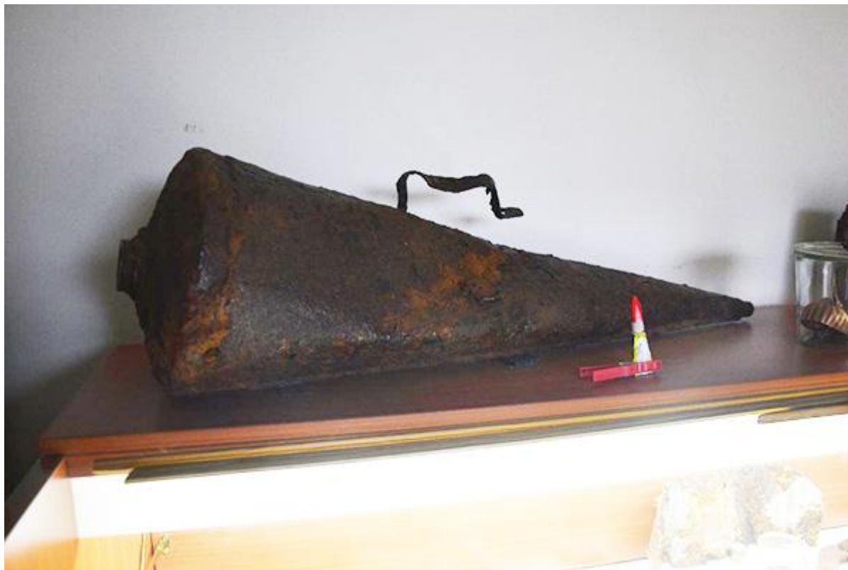
PS: It's a Minimax fire extinguisher!
