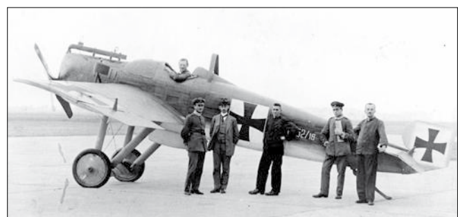
Junkers J.2 E.252/16, a development of the J.1, slightly smaller and of cleaner appearance. This was the third of five (total) of the type built. It was fitted with a 160hp Mercedes D.III engine. :CCI Archive
