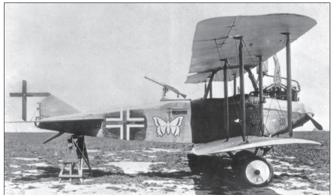
DFW C.V 287/18 as captured, with its Parabellum gun fitted and showing both the fuselage butterfly marking and the style of its national markings. The darker background to the fuselage cross was probably applied to mask the original Maltese cross. :Greg vanWyngarden
