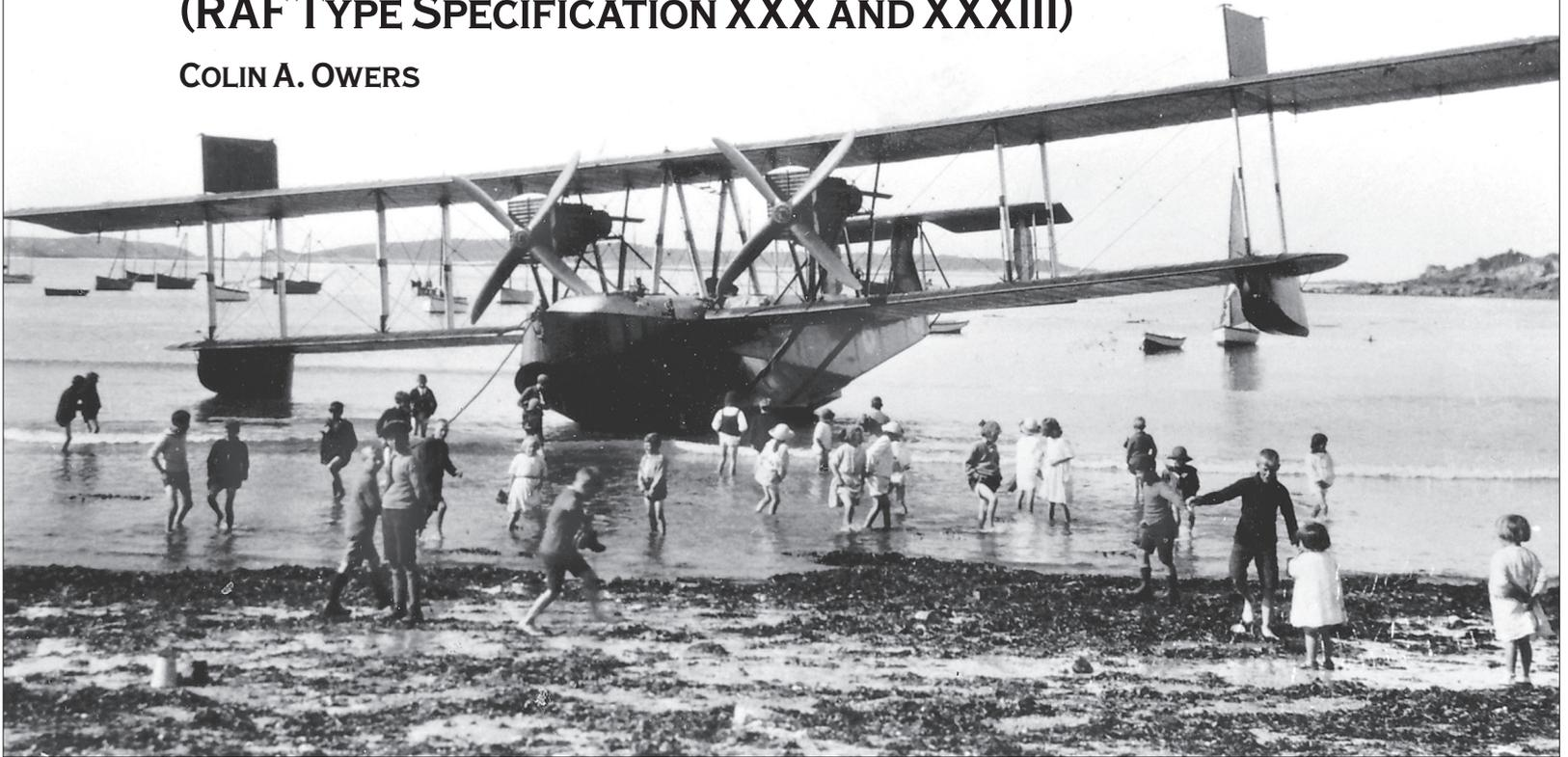
Above and Below: N120 after the hull was holed in shallow water at St Mary's, Scilly Isles. The airscrews were taken from the wrecked Vickers Valentia N124.
