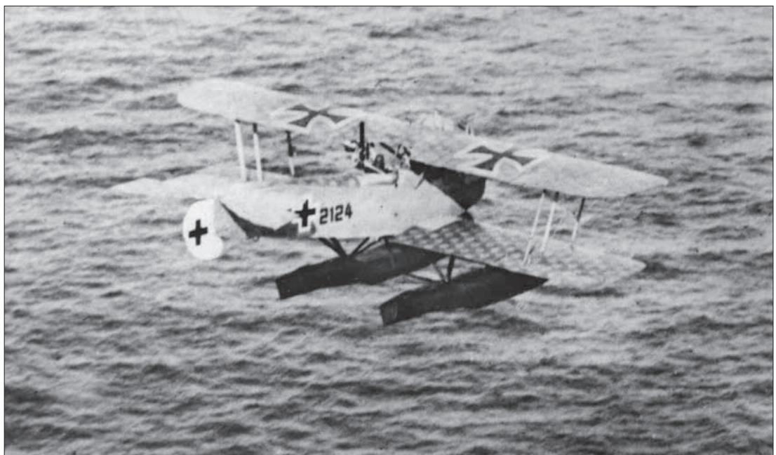
Late model Hansa Brandenburg W.12, serial 2124, in flight over the sea. The effectiveness of the hexagonal camouflage pattern is noticeable on the lower wing. : CCI Archive
